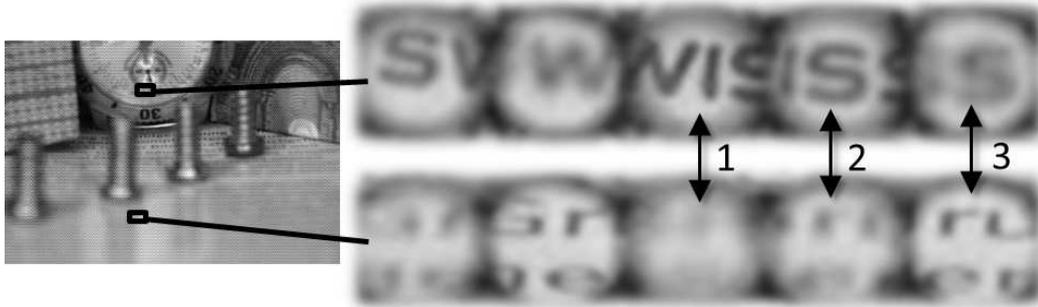
Figure 12. Effect of different micro lens focal lengths on the micro images formed for different object depths. 1, 2 and 3 indicate the different micro lens types.
